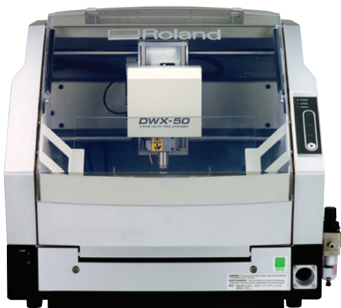
Figure 14. The Roland DWX 50 is a 5-axis machine more than capable of milling most materials. Perfect to mill PEEK!
